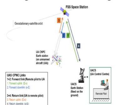
Links 1 and 4 are at fixed specific location and consistent with regular FSS operation. Links 2 and 3 involve mobile earth stations and require additional consideration
